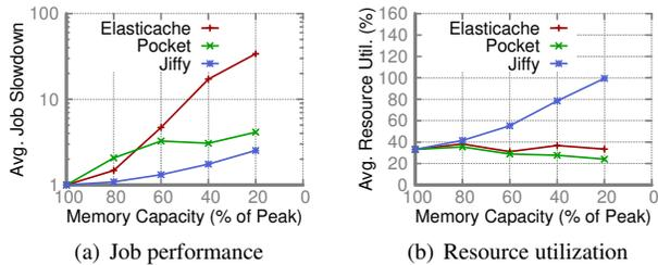
**Fig. 9. Fine-grained task-level elasticity in Jiffy** enables (a) better job performance, and (b) higher resource utilization under constrained capacity. In (a), the slowdown is computed relative to the job completion time with 100% capacity (for this data point, Elasticache performance was 30% worse than Pocket, and Pocket performance was 5% worse than Jiffy). See §6.1 for details.
