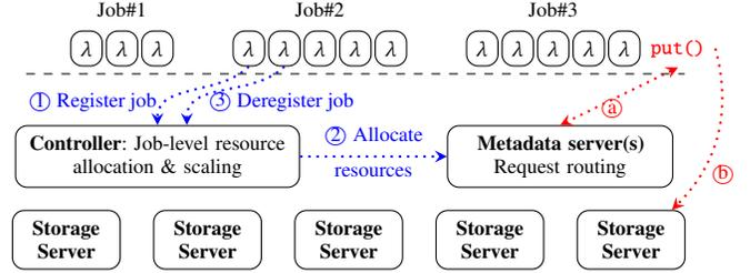
**Fig. 2. Pocket Architecture.** Steps ①–③ show how jobs are registered, resources are allocated and jobs are deregistered, while ④, ⑤ show how operations are routed from serverless compute tasks to servers in the data plane via metadata servers (Fig. adapted from [8]).
