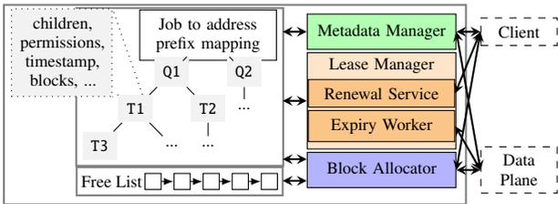
**Fig. 7. Jiffy controller.** See §4.2.1 for details.
