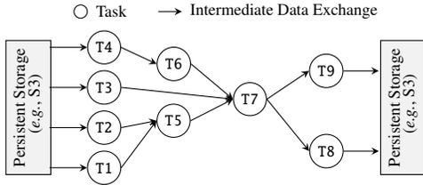
**Fig. 3. Execution DAG example for a typical analytics job.** Intermediate data exchange across tasks occurs via Jiffy.
