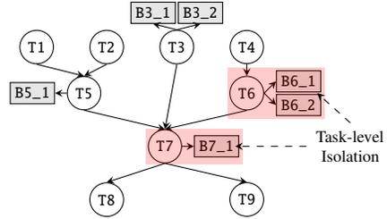
**Fig. 4. Hierarchical addressing** for the job in Fig. 3. Jiffy provides task-level resource isolation for far-memory under each task address-prefix (§3.1). Note that block addresses are only assigned to address-prefixes with currently allocated blocks; for tasks T1, T2 and T4, blocks are not stored in Jiffy, but read from persistent storage.
